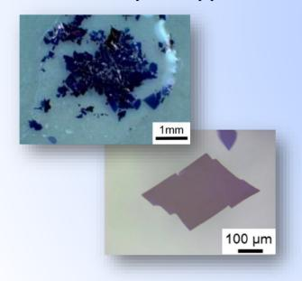
Some organic compounds such as pentacene and fullerene exhibit a semiconducting conductivity. The single crystal of such organic semiconductors is usually obtained by a solution growth method, as is daily seen in the crystallization of "salt crystals" from a saturated saline solution.
