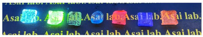
Various luminescence color (wavelength) can be obtained by using various metal ions as "luminescent centers".
