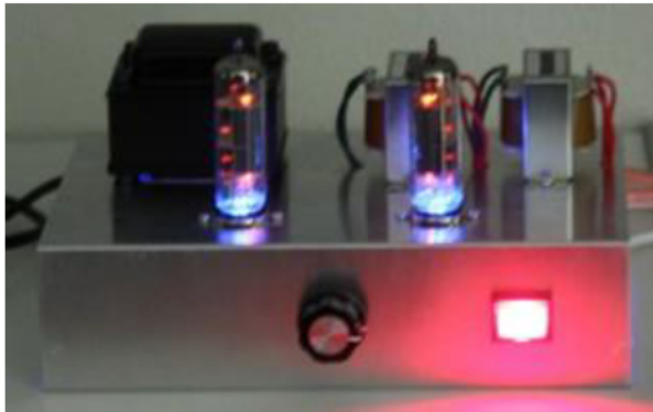
An example of audio amplifier with vacuum tubes
