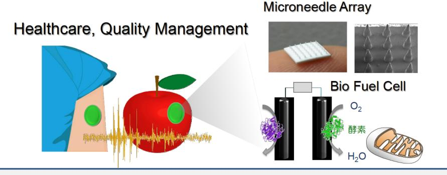
Students will experience the fabrication of a biosensor patch by using a microneedle array and/ or enzymatic biofuel cells. The water and sugar content in fruits will be measured by the fabricated sensor patch.
