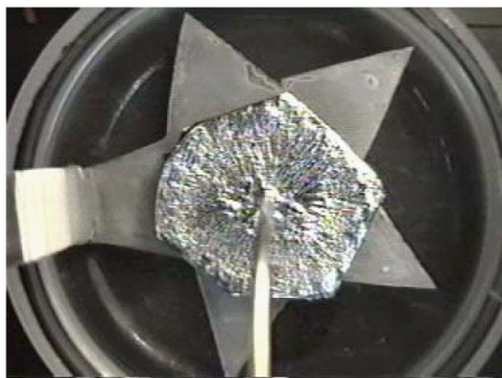
Fig. 1 Metal Leaves produced with a star-like electrode.
