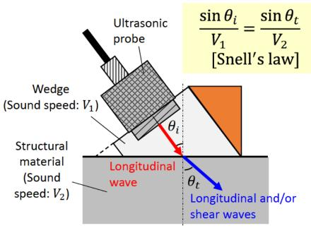
Ultrasonic nondestructive inspection (angle beam method)
