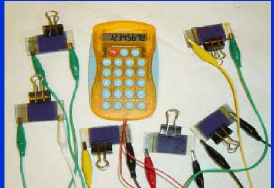
A calculator driven by dye-sensitized solar cells
