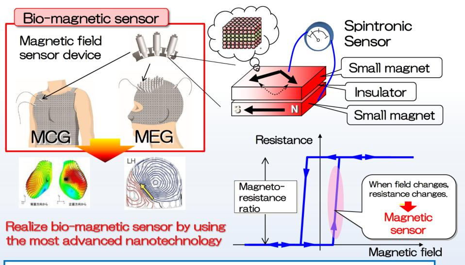
We will learn how to fabricate magnetic sensor, and try to measure the weak magnetic field from human heart, environmental magnetic noise, small defect in steel etc.
