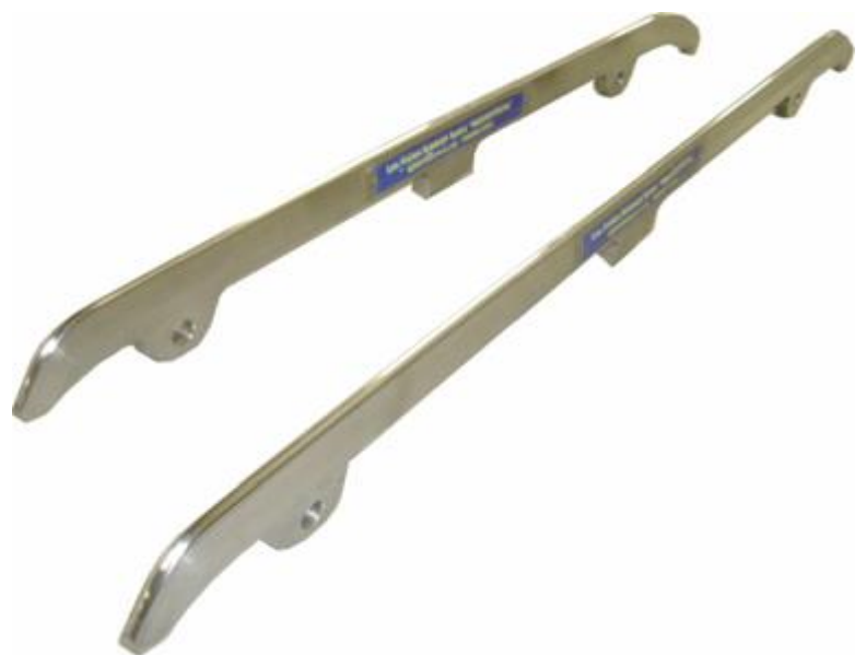
Low friction bobsled runner " NAGANO SPECIAL " which was used in Nagano Olympic Winter Game in 1998.
