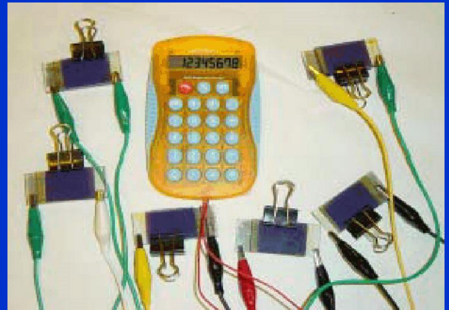
A calculator driven by dye-sensitized solar cells
