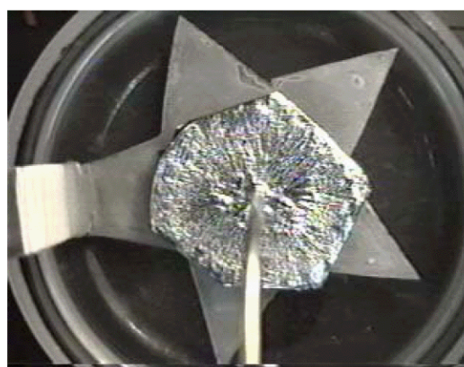
Fig. 2 Metal Leaves produced with a starlike electrode.
