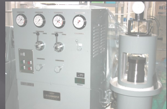
Equipment for hydrostatic bulge testing
